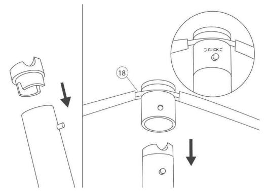
6. Assemble the TOP FITTING (netting support) as shown in the image below.
