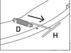
6. Install and stretch the remaining springs. Do not move the trampoline until assembly is complete.
