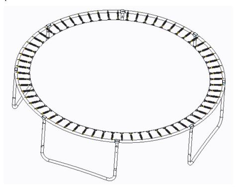
7. Cover the springs using the pad .Attach the pad to the springs using the elastic straps.
