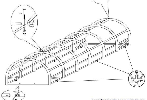
Loosely assemble complete frame, before tightening all bolts in final position.
