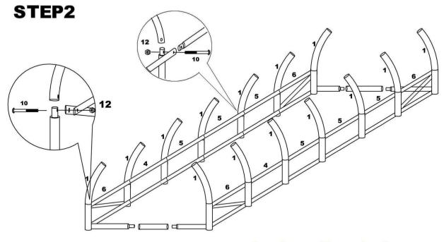
Loosely assemble complete frame, before tightening all bolts in final position.
