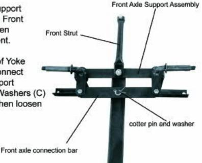
Attach Front Axle Support Assembly to front of Bed using M8 x 20 Carriage Bolts (H), M8 Washers (C) and M8 Nylon Nuts (D).
